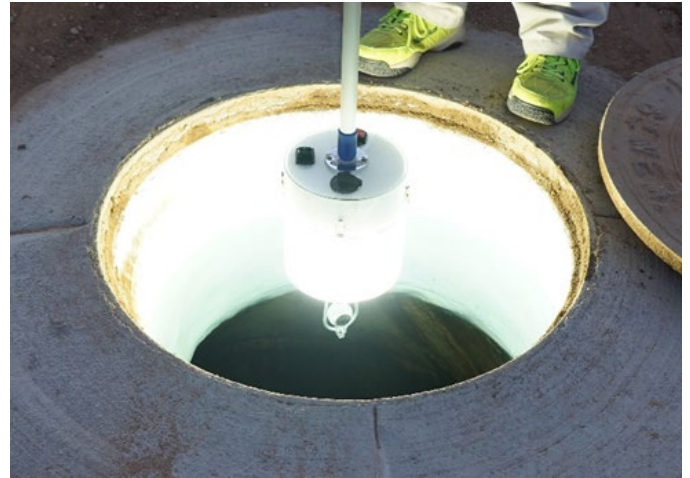
Pole Camera Equipped with LED Lights for Visibility
