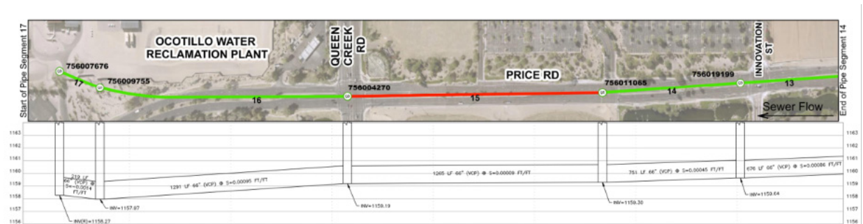
Figure 2 - 66-inch Sewer Profile
